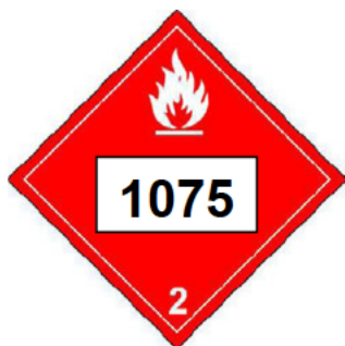
Figure 2: TDG Placard for Liquefied Petroleum Gas (LPG)
